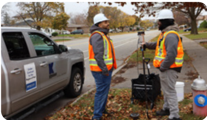
Field engineers conduct a non-invasive Dynamic Response Imaging™ (DRI™) survey for The Region of Peel, gathering critical pipeline condition data without service interruption.
