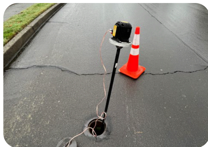
KenWave's DRI system in action: a vibration generator introduces vibroacoustic signals into the pipeline to assess structural integrity—all without excavation. Photo taken during the Gresham, OR pilot project.
