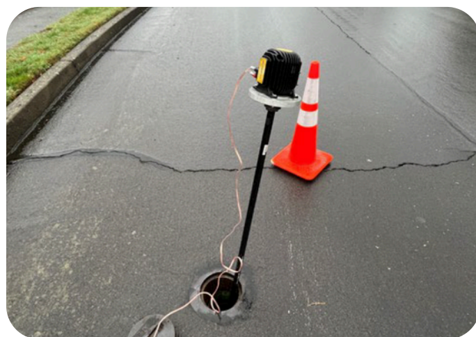
KenWave's DRI system in action: a wave generator introduces vibroacoustic signals into the pipeline to assess structural integrity—all without excavation. Photo taken during the Gresham, OR pilot project.
