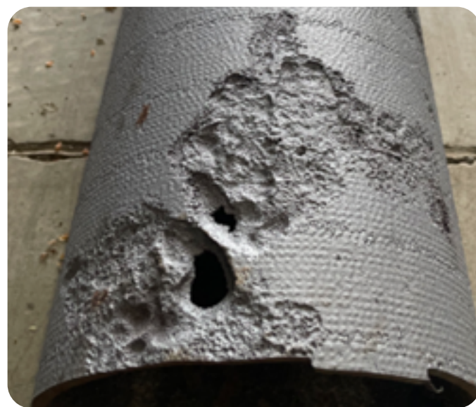
Validation of KenWave DRI technology showing at location 1 distress on a section of ductile iron pipe.
